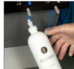
Insert RinseAway into the 3rd port, open the toggle and perform a 20-second system rinse
