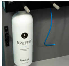
Insert RinseAway into the 1st port, open the toggle and perform a 20-second system rinse
