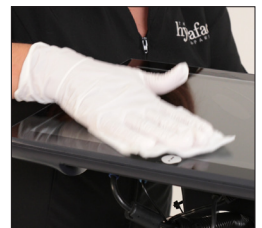
Use a glass cleaner and a microfiber cloth or towel to clean the system touch screen Spray on the cloth, not directly on the screen
